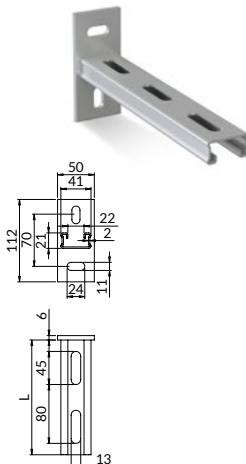
**Usage:** universal channel system for building fastening systems, with repeatable perforation and serrated edges in order to lock the accessories better; they have a cut centimeter scale on the channel side.
