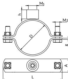
**Usage:** Temperature differences cause pipes to decrease or increase in size and cause installations to move. By using fixed (and sliding) points we can guide the pipe movement in the desired direction - thus protecting the installation from damage. Properly designed placement of fixed points guarantees trouble-free operation of the installation.
