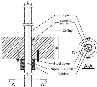
Fig. Passage of cables in PVC pipe through ceiling protected by a Nipro ECG collar.
