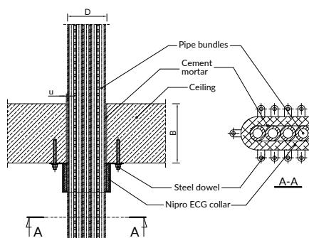
Fig. Passage of a bundle of five combustible pipes through the ceiling secured by a single Nipro ECG collar.
