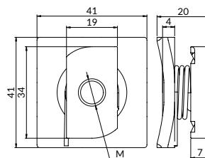
**Usage:** for fastening accessories in the channels and in the cantilever arms; compatible with channels and cantilever arms; a finished element with a washer and a spring; a compact solution which ensures quick assembly; multi-part element assembled, ready for use.
