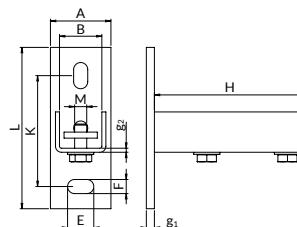
**Usage:** connection of channels with the base material; allows independent creation of channels with feet and construction of fastening systems.
