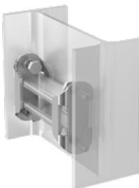
**Usage:** for use with MF profile; installation inside the channel or I-section with 4 expansion bolts; After tightening the bolts, additionally counter them with a nut; The length of the MF profile should be cut to the internal dimension of the girder.
