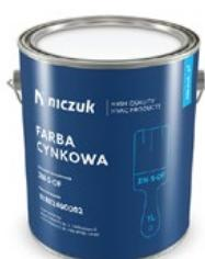
**Usage:** repair of damages of zinc layer and anti-corrosion protection of products made of carbon steel in the places of cuts; paint of high zinc content; for repairing and renovating joints, damaged places on the zincplated surface; it contains 90% of zinc in the form of metallic dust; resistant to 300°C; it has excellent anti-corrosion properties in contact with atmospheric conditions.
