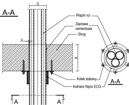
Fig. Passage of a bundle of three combustible pipes through the ceiling secured by a single Nipro ECG collar.
