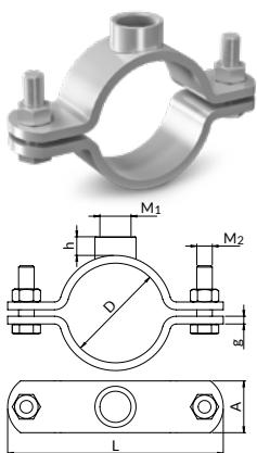
**Usage:** for taking over forces resulting from pipeline elongation and directing the elongations in the desired direction.
