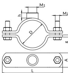
**Usage:** for taking over forces resulting from pipeline elongation and directing the elongations in the desired direction.
