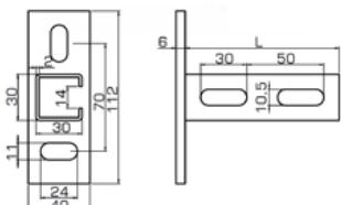
**Usage:** universal channel system for building fastening systems, with repeatable perforation and serrated edges in order to lock accessories better; with cut centimeter scale on the channel side.
