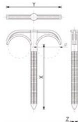
**Usage:** intended for fixing and laying pipes with the external diameter of up to 32 mm. Possibility of setting in the floor made of concrete of class not lower than C16/20. The shape of the mandrel ensures easy and quick assembly in the insulation layer at the same time guaranteeing stabilization of pipes laid during the screed realization.
