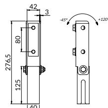
**Usage:** A complete element connecting profiles with a width of 41mm with the PDT roof support, intended for creating frame structures from rail profiles, for installations or devices.
