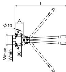
**Usage:** for performing openings in trapeze metal sheets; there are two types of pliers available with the maximum jaw opening up to 105 mm and up to 145 mm; they ensure speed of operation, time saving.
