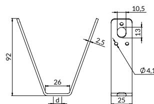
**Usage:** For quick installation of all types of installations and air duct suspensions. With the WT-BK hanger it is possible to suspend various elements to the roof structure made of trapezoidal sheet metal, using self-drilling screws, threaded rods or screws.
