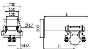
Fixed point clamp of PSF type welded to the installation kit (clamp data are specified on [page 65](#)).
