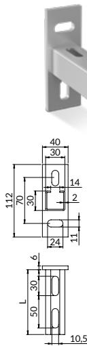
**Usage:** universal channel system for building fastening systems, with repeatable perforation; with cut centimeter scale on the channel side.
