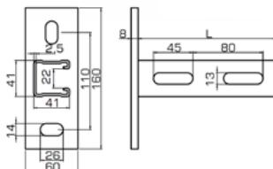
**Usage:** universal channel system for building fastening systems, with repeatable perforation; with cut centimeter scale on the channel side.
