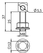
**Application:** for mounting elements with 8 mm holes (luminaires, mounting channels, cable ladders). The steel wire rope is interlaced through the hole in the adapter.
