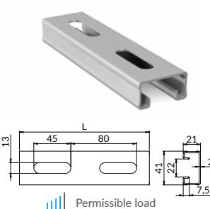
**Usage:** universal channel system for building fastening systems; with repeatable perforation and serrated edges in order to lock the accessories better; they have a cut centimeter scale on the channel side.
