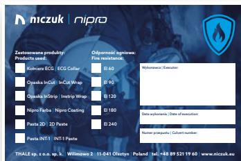
**Usage:** Plaque to be completed with information on passive fire protection: fire resistance class, name of contractor, date of construction, system used. To be placed in a prominent position next to the fire-protection culvert.
