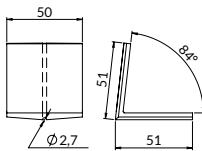
**Application:** prevents the steel wire rope from rubbing against the edge of the ventilation channel.
