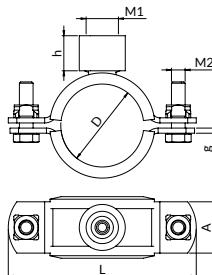
**Usage:** Temperature differences cause pipes to decrease or increase their dimensions and cause the installation to move. By using fixed (and sliding) points, we can guide the movement of pipes in the desired direction - thus protecting the installation against damage. Properly designed arrangement of fixed points guarantees failure-free operation of the installation. The lining protects pipelines against mechanical damage and additionally provides vibration damping.
