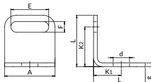
**Usage:** for structural connection of pipe clamps; for fastening risers while fastening behind the pipe clamp side opening.
