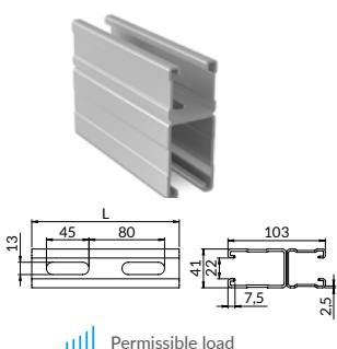
**Usage:** universal channel system for building fastening systems, with repeatable perforation and serrated edges in order to lock the accessories better; they have a cut centimeter scale on the channel side.
