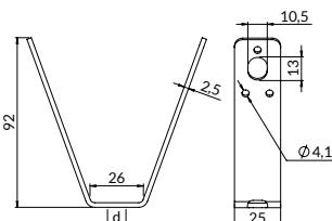
Usage: assembly of fixed water extinguishing devices to trapeze metal sheets.
