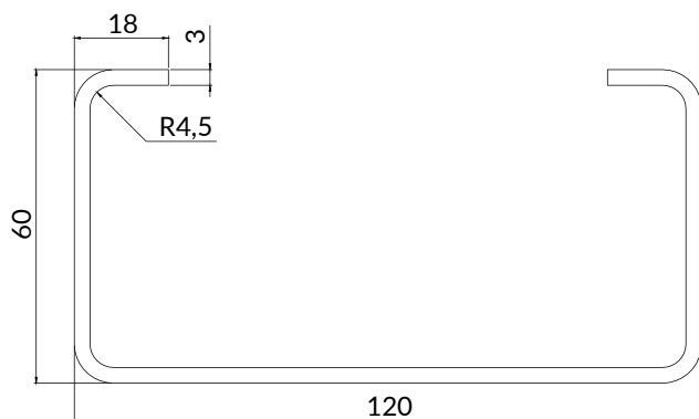
Fig. 1-1 Cross-section of VS3H pole
